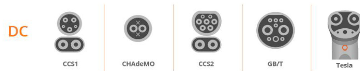
Figure 7. Fast DC Charger Connector Types. Tesla uses a proprietary connector in North America and other regions. In Europe and other regions where CCS and CHAdEMO networks are deployed, Tesla is adapting to these systems. Source: EnelX
